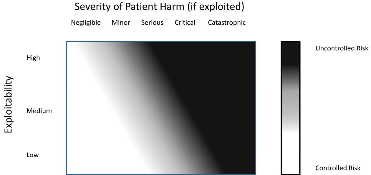
Figure – Evaluation of Risk of Patient Harm. The figure shows the relationship between exploitability and severity of patient harm, and can be used to assess the risk of patient harm from a cybersecurity vulnerability. The figure can be used to categorize the risk of patient harm as controlled or uncontrolled.
